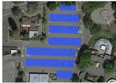
Bech Parking Lot Helix Array Layout – 878kWdc
